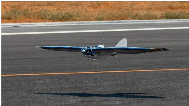
Birds can be a great danger to aircrafts in airport. For this reason, we have developed a UAS shaped like a bird that allows to control the wildlife in the surroundings of an airport quickly and efficiently.
